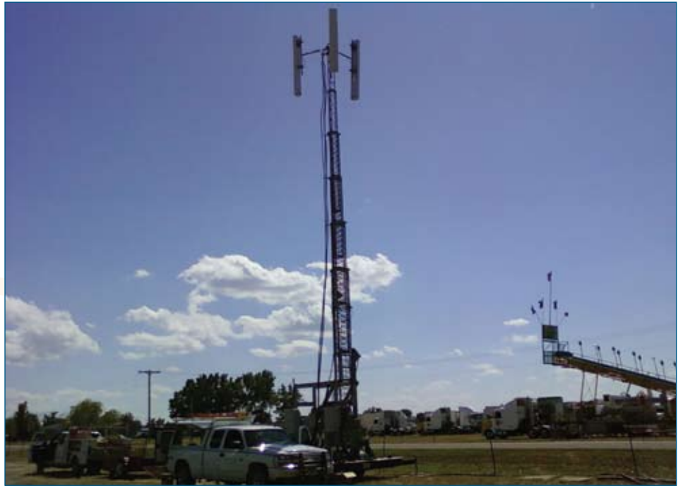
Nemont's Cell on Wheels (COW) was first deployed at the Wolf Point Wild Horse Stampede in July to help alleviate problems caused by higher-than-normal call volume.
